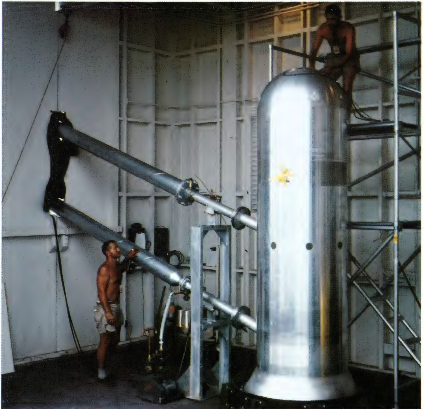
FIGURE 7-33. TEWA DEVICE (D-3, HOB = 8 2' ABOVE WATERLINE)
